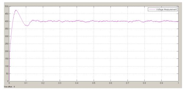
Figure 4 Output voltage (V<sub>0</sub>=400.3V).
