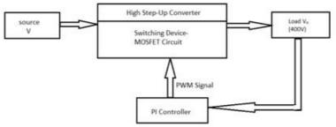
Figure 1 Proposed block diagram
