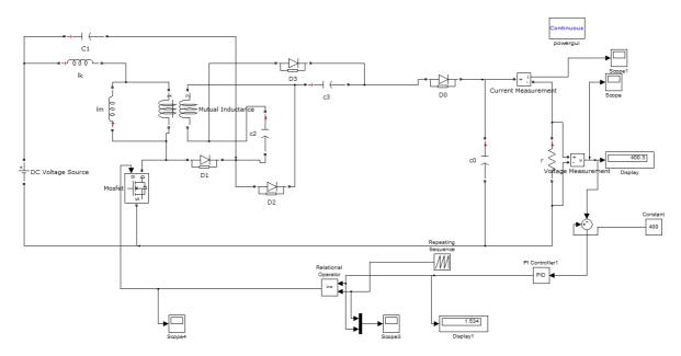
Figure 3 MATLAB Simulation Diagram of proposed converter with PI controller.
