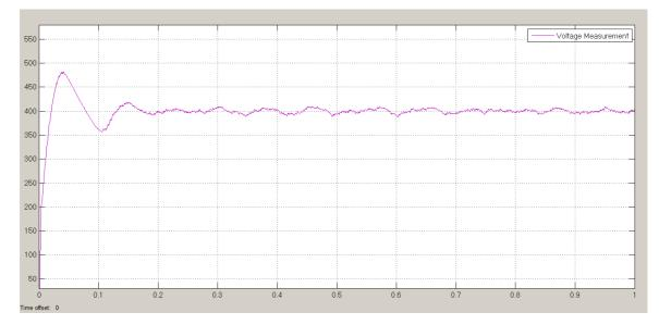
Figure 7 voltage waveform for the values  $K_P$ =0.009 and  $K_I$ =1.5.
