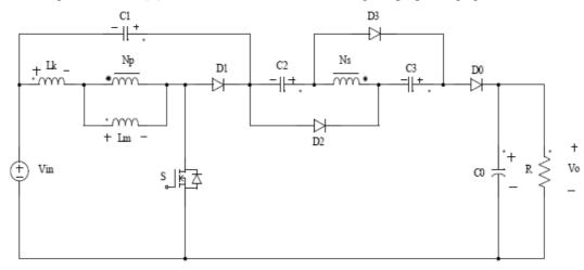
Figure 2 Circuit configuration of the proposed converter
